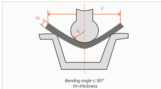
The bending force depends on UTS plate thickness, bended length and die opening V.
