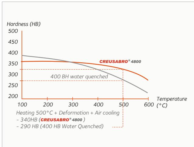
These properties enable the steel to be processed in the hot condition 450 - 500 °C (840 - 930 °F): forming of thick plates, for example, followed by a slow cooling without inducing any significant drop of hardness. Hot resistance of Creusabro® 4800 allows its use in hot environments where pieces are heated up to 350 °C (660 °F).
